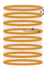
**FIG.1:** A piezo stacked transducer made of N circular (radius R) superconducting turns, embedded in a piezoelectric ceramic.
